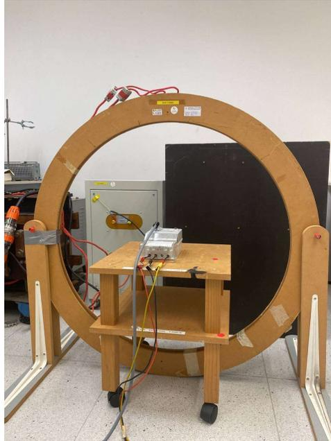
**Figure 36: Magnetic Induction Setup (F-B)**
