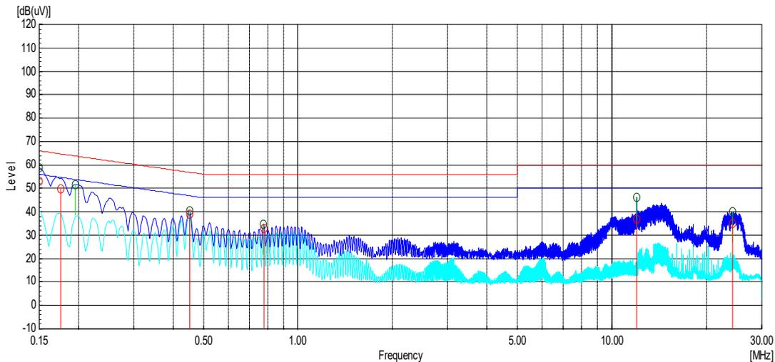
Table 30: Radio Frequency Conducted Emissions Test Results - Meter SN934 (Line 1)
