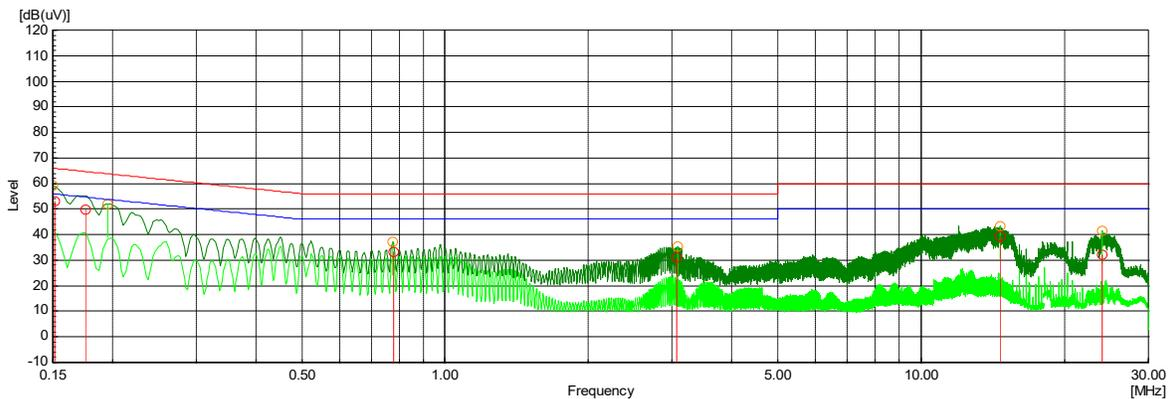
Table 31: Radio Frequency Conducted Emissions Test Results - Meter SN934 (Neutral)
