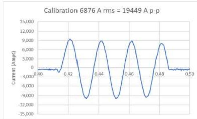
Figure 3. 7 kA Calibration
