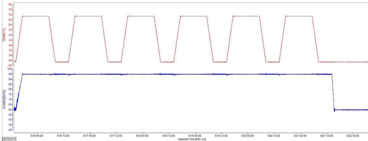
**Table 7: Impulse Test (after damp heat cyclic) Test Results**
