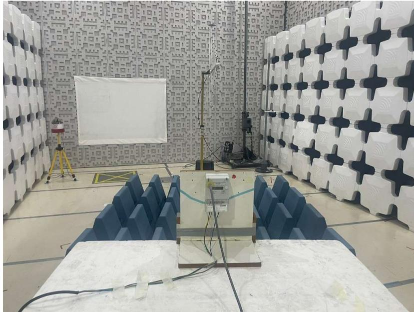
**Figure 16: Immunity to electromagnetic RF fields Test Setup (10V/m) 1-2.4GHz**
