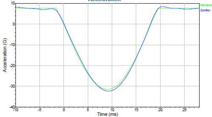
**Figure 7: Shock Test Plot S-S (+)**
