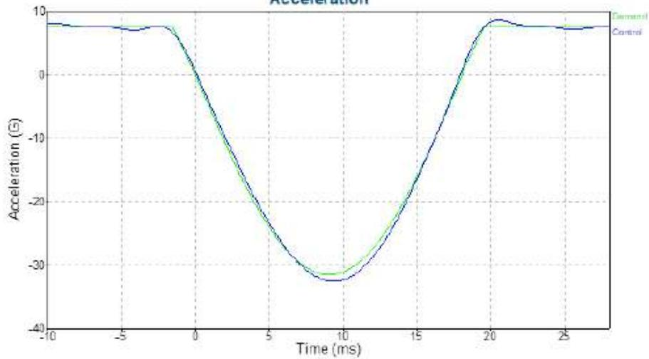
Figure 5: Shock Test Plot F-B (+)
