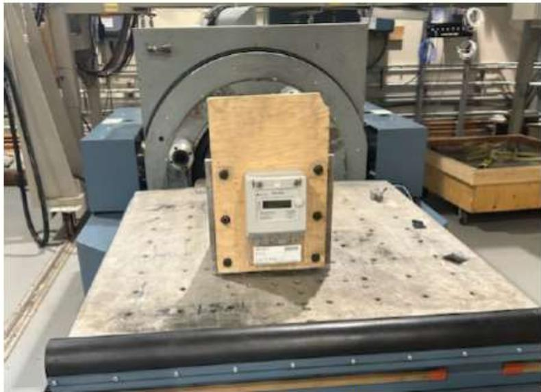
Figure 2: Shock Test Configuration (S-S)
