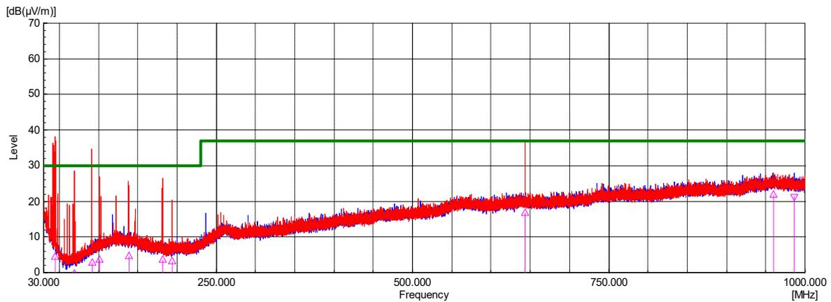
**Table 32: Radio Frequency Radiated Emissions Test Results - Meter SN934**
