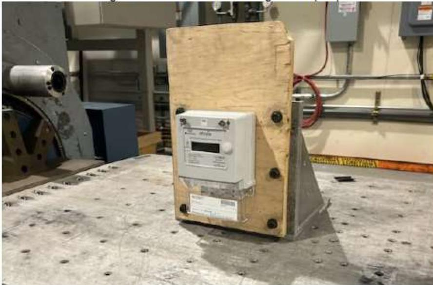
Figure 12: Vibration Test Configuration (V)
