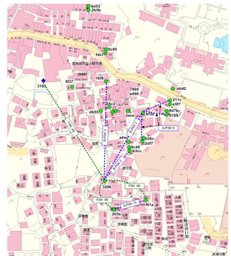
Figure 17 – Multiple PLC and RF Links (not all links shown)
