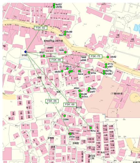
Figure 16 – Visibility from the Field Area Router (not all links shown)
