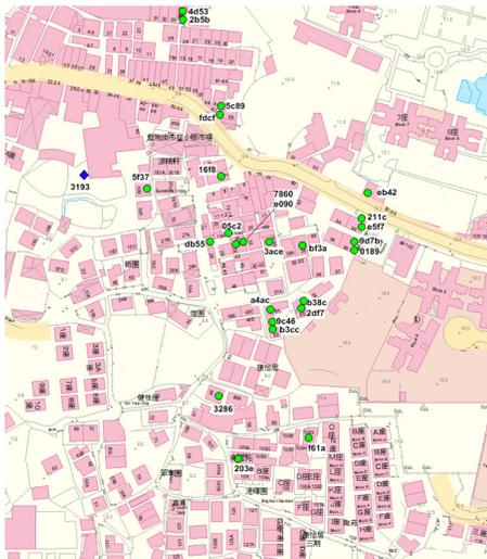
Figure 15 – Village Meter Installation Layout
