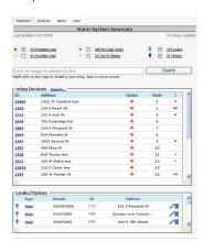
Leak Sensor+ information table displays all Leak Sensor+ data from one or more water distribution systems—sorting, searching and ranking all sensors by leak status:
